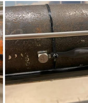
Accelerometer reference probes
